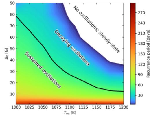
**Figure:** Thermoresistive instability domain. Y-axis is the radial magnetic field strength instead of pressure. Taken from Hardy et al. 2023.
