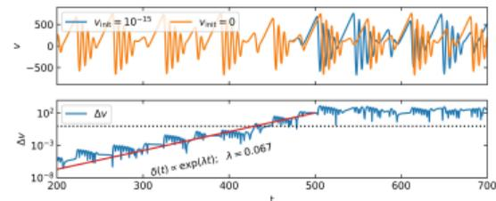
Figure: Decorrelation between unperturbed and perturbed solutions with the associated Lyapunov coefficient.
