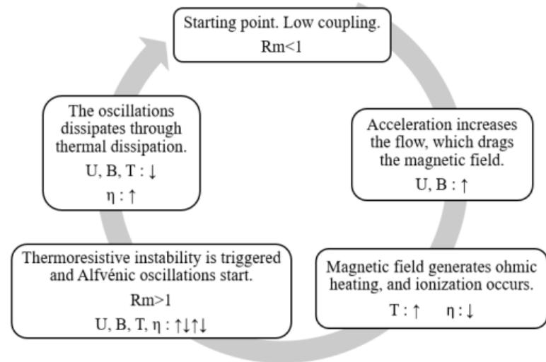
**Figure:** Flow chart of the instability workings. The oscillation between low coupling ( $Rm < 1$ ) and high coupling ( $Rm > 1$ ) between the field and flow is key.
